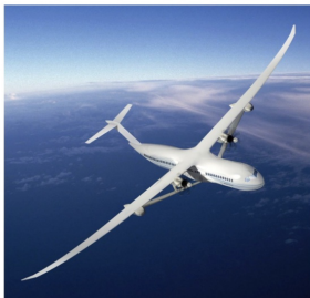
NASA Transonic Truss-Braced Wing
