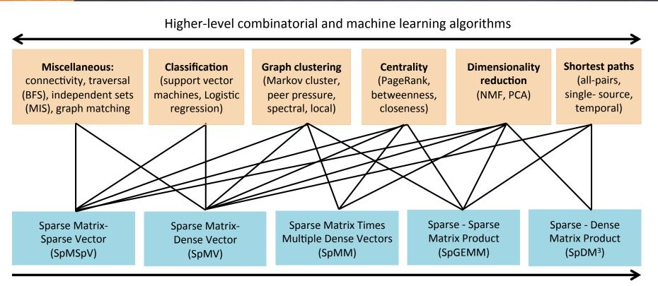
GraphBLAS primitives in increasing arithmetic intensity
